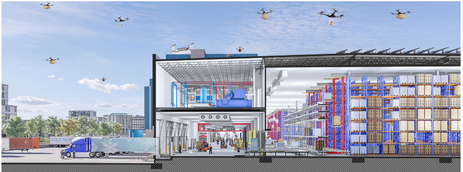
Figure 3.12 Lowered dock roof with double column line.
