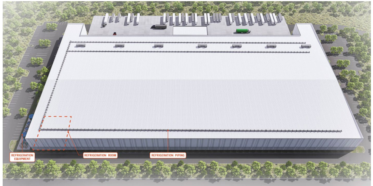
Figure 3.2 Refrigeration equipment placement on rear of building and parking in front.
